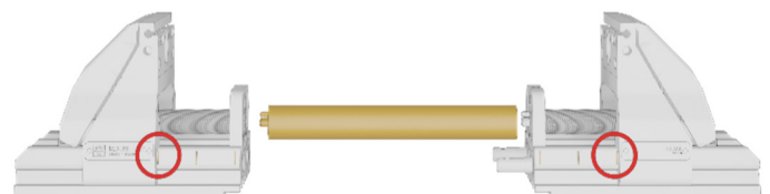
Fig. 28: Inserting the adjusting spindle extension
