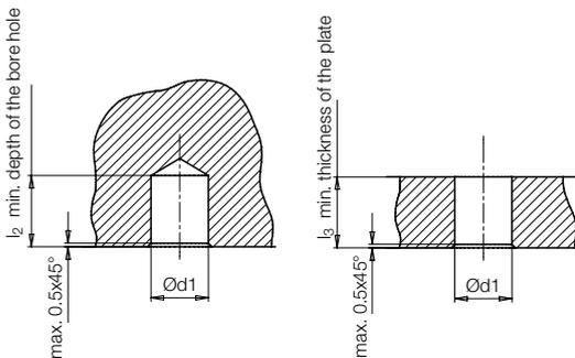
Adjusting  $\varnothing$  of the clamping bushing:  $k = d1 - 0.2$  mm
