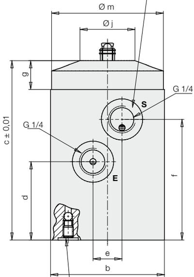
For manifold mounting remove stud screw with ball and insert O-ring into the counterbore (see accessories)
