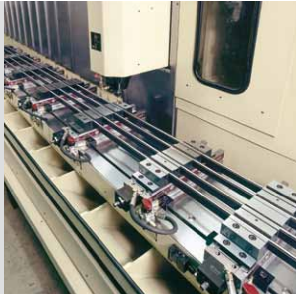
DS hydraulic with floating jaws
