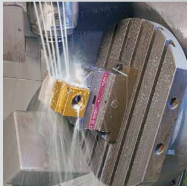
MC for 5-sided machining
