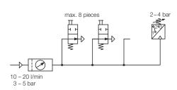
For the evaluation of the pneumatic pressure build-up, standard pneumatic pressure switches can be used. It is possible to monitor with one pressure switch up to 8 position monitorings connected in series (see circuit diagram). It has to be considered that process-safe functioning of pneumatic position monitorings is only guaranteed with throttled air and system pressure. The nominal values are indicated below technical characteristics.
