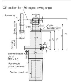
Clamping arm can be fixed in any desired position.
