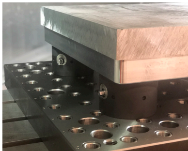
Four Drop Zeros mounted on a Carr Lane Mfg. modular fixturing plate holding an aluminum billet part.
